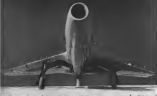
AMERICINI SAGITTARIUS is at all-ward construction and features nose intake for its single 300 lb. thrust Turbomeca Marboré turbojet. Note plane's wing braces.
